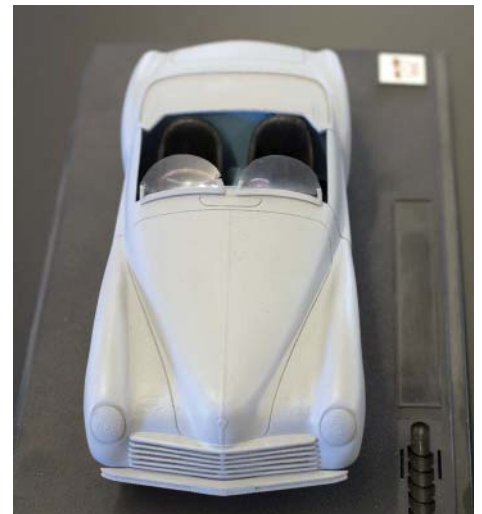
Front view of the 3D-printed, 1/12 scale resin model, built to show the car's actual shape and to verify the digital renderings.
