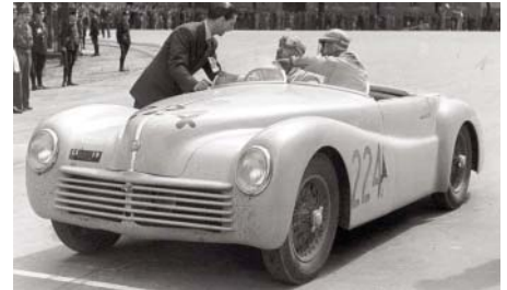
For the 1948 Mille Miglia, the Alfa's bumpers, front windshield, convertible top, and side windows were removed, and Brooklands style racing windscreens were installed.
