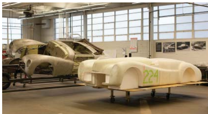
The finished buck shown next to the body, which is mounted on a rotisserie fixture in Cooper Technica's Chicago studio.
