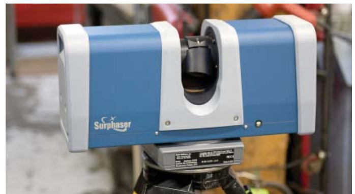
The laser scanner is positioned at various points around the car to capture a 360-degree digital image of the body and chassis.
