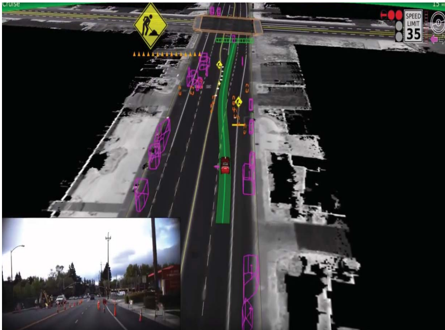
The Google car's "brain" in action, as it weaves together data interpreted by its cameras, as well as other sources, to navigate through a construction zone.
