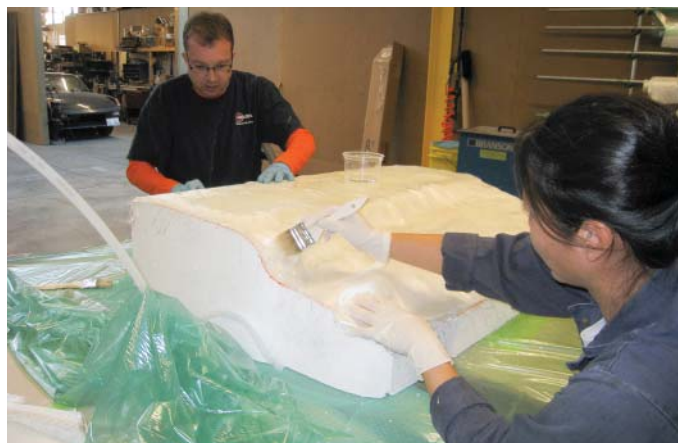
Applying the fiberglass and resin to the bucks.
