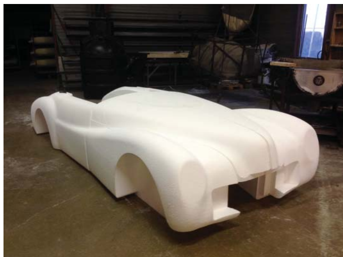
The bucks were individually machined on a 5-axis milling machine and test-assembled into the full-size body shape.
