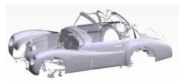
Raw laser scan image of the 1943 Alfa Romeo 6C2500 (photo courtesy of Cooper Technica Inc.)
