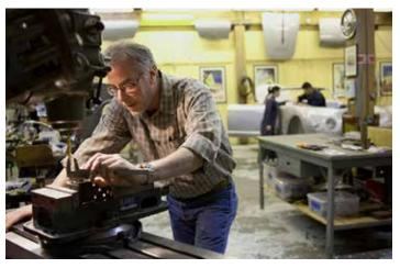
David at work - measuring before drilling on the Bridgeport milling machine (photo courtesy of Cooper Technica Inc.)
