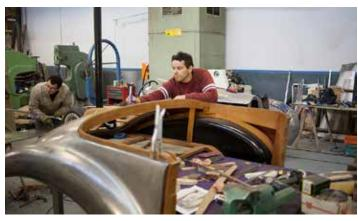
Fitting the trunk panel on the restored rear body section of the 1948 Delahaye at the shop in France (photo courtesy of Cooper Technica Inc.)
