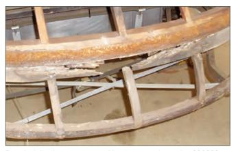
Detail of the damage sustained by the original wood in 800858. The wood supporting the trunk has cracked and rotted. This wood cannot be repaired safely or effectively by splicing and impregnating the wood with resin. (*David Cooper*)
