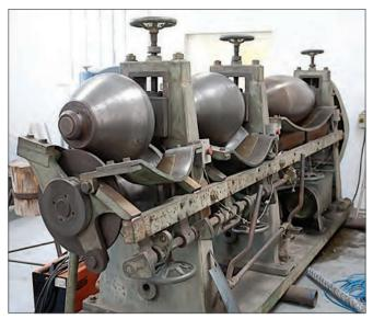
French Crown Forming machine, also known as the Three-Olive machine. This particular machine, now restored and in use at Cooper Technica's workshop, was originally owned by Henri Chapron. The machine weighs approx. 3,175 kg and is 3.2 m long. (*David Cooper*)
