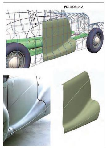
Detail of the digital rendering of the right door of 800858. The original door is shown in the lower left for comparison with the rendering. The rendering forms the basis for fabricating new body *maquettes* for the sheet metal panels. This allows the original sheet metal door panel to be restored exactly to its correct dimensions. It eliminates distortions introduced in previous repairs. (*David Cooper*)
