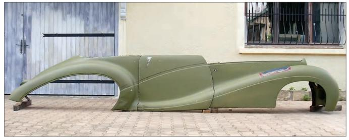
Side view of the original sheet metal panels of Delahaye 135M 800858 after removal from the body. These panels were in excellent condition and over 85% could be preserved and reinstalled. (*David Cooper*)
