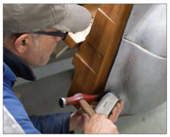
Installing the rear body sheet metal of 800858 around the wood skeleton at the door panel. The sheet metal is wrapped around a steel edge screwed to the wood door jamb support. (*David Cooper*)
