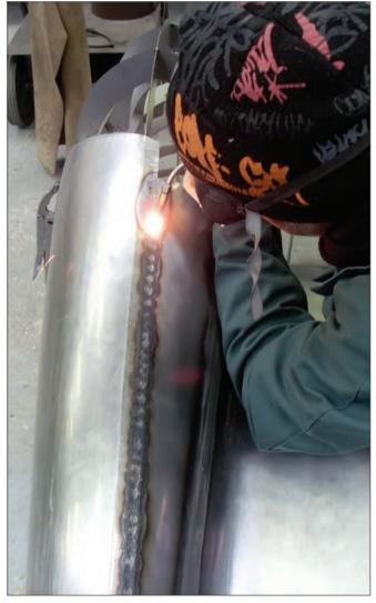
Butt-welding two panels together on a fender by hand using a gas or oxygen-acetylene torch. Note the narrow band of coloration change showing the limited heat used in this type of welding. (David Cooper)
