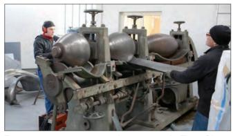
Two operators are necessary to form parts on the Three-Olive machine. The machine can be powered in either direction, but does not feed the part. One metal shaper locates and feeds the part in the right portion of the roller to achieve the desired arc. The other man pulls the part through the machine, twisting it to the side if a compound curve is desired. (*David Cooper*)
