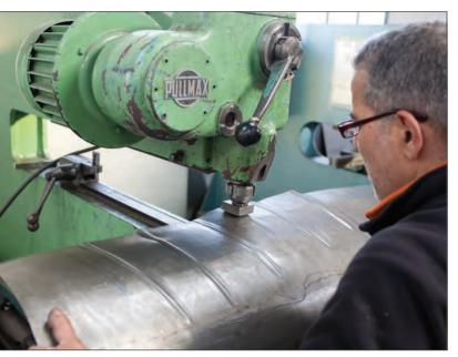
Forming darts on a Pullmax for shrinking the sheet metal along an edge, without affecting the dominant curve on the sheet metal panel. Pullmax tools are made by the metal shaper for the effects he desires. (*David Cooper*)
