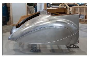
Rear body of 800858. Note the sweep of the curve across the rear wheel skirt. Saoutchik accented this curve by swaging the body panel below the curve. He then installed a chrome panel over this embossed section, not shown here. (*David Cooper*)
